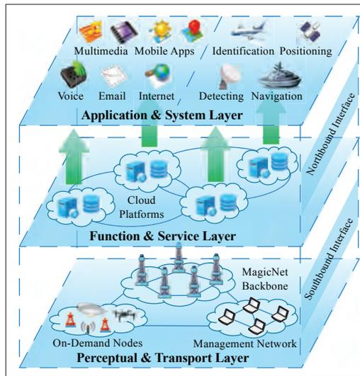
FIGURE 3. The three-layer software-defined architecture of the MagicNet.
