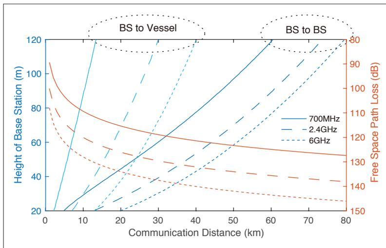
FIGURE 2. The required BS antenna height based on Fresnel zone model and free space path loss vs. communication distance.
