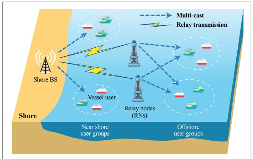
FIGURE 4. The structure of the near-shore multicast relaying system.
