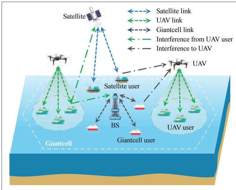
FIGURE 5. The structure of satellite-UAV-giantcell three-tier hybrid network.
